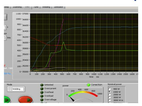
There is an inserted function for **recording data** – frequency, output current, phase, amplitude, power and PWM. Select the duration of the record in the field "**Sampling time**" – in seconds. The recording starts by START of the generator and ends when the selected time to write is finished. After recording is finished, when the button read is pressed, the data from generator is uploaded in the Labview software and is visualized graphically.
