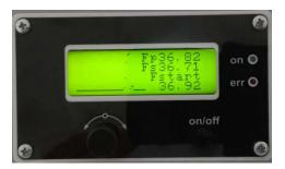
After pressing the ON/OFF button, the generator scans at a low power in the interval from fstart to fstart-scanning range(you can set scanning range only in the Labview software). If in this interval persists ultrasonic resonant load, than the generator shows it's parallel frequency fp and serial frequency fs. It also shows recommended fstart on the bottom(which is fp + 100 Hz).
