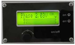
Here you can see and set the operating phase. To edit the value of the phase, you need to push once the encoder knob and by turning left or right adjust the value of the starting frequency. After pushing the knob you will notice that the letter "v" over the right corner of the dynamic bars will become "j".
