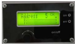
Here you can see and set the operating Modbus address. To edit the value of the address, you need to push once the encoder knob and by turning left or right adjust the value of the starting frequency. After pushing the knob you will notice that the letter "v" over the right corner of the dynamic bars will become "j".
