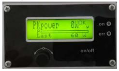
"<u>Welding by limiting the Peak power on the load</u>". Welding process will stop when Peak power is reached.
