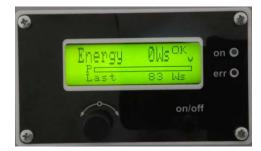
"<u>Welding by limited amount of Energy</u>" which should be sent to a load. Welding process will stop when given amount of Energy is delivered to a load.
