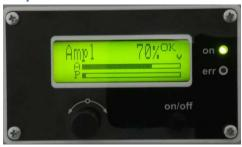
Display shows the set value of output amplitude(output voltage) and its performance on "A" bar. From 0% to 100% of nominal output amplitude. During initial testing of new sonotrodes, set the amplitude to some low value (example: 50% to 60%).
