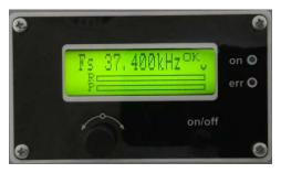
Here you can see and set the initial operating frequency. To edit the value of the frequency, you need to push once the encoder knob and by turning left or right adjust the value of the starting frequency. After pushing the knob you will notice that the letter "v" over the right corner of the dynamic bars will become "j".
