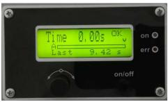
Welding process will stop after given Time interval.
