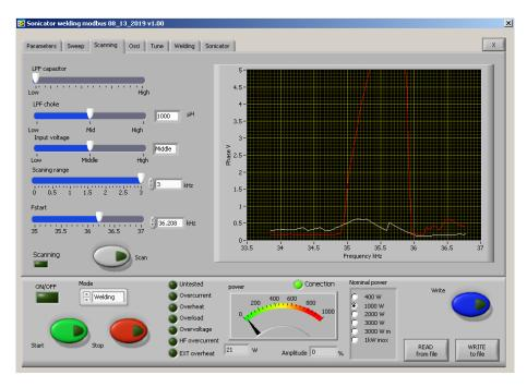
The generator has Scanning function which is very powerful instrument for the operator. Here you can discover the phase and current characteristic of the exact load. It is shown graphically in a window in Scanning tab.
