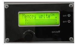
To save all parameters or changes in the EEPROM of the generator, you need to push once the encoder knob and by turning left or right memorize all settings. After saving is done the initial window **Start Frequency** appears . After pushing the knob you will notice that the letter "v" over the right corner of the dynamic bars will become "j".
